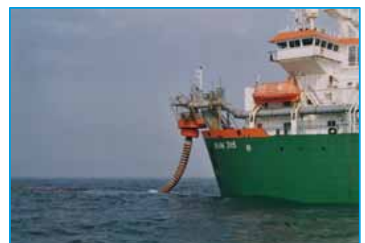
Dredge Ham 316: Connection operation between the dredge and the floating pipeline
