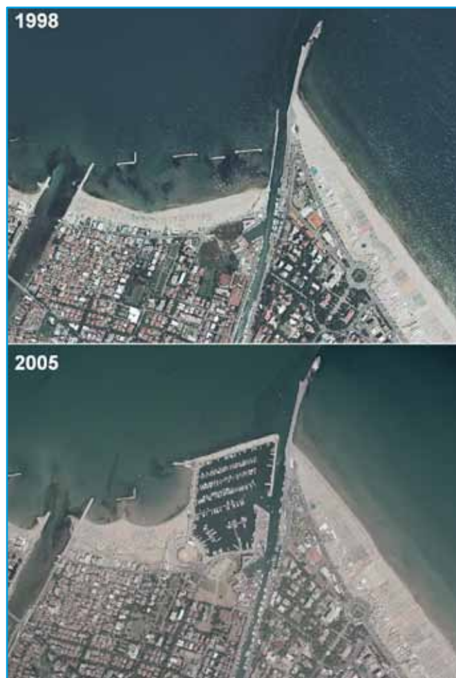
Figure 92 - San Giuliano Beach, before and after the construction of new marina near the pier north of the port canal.
