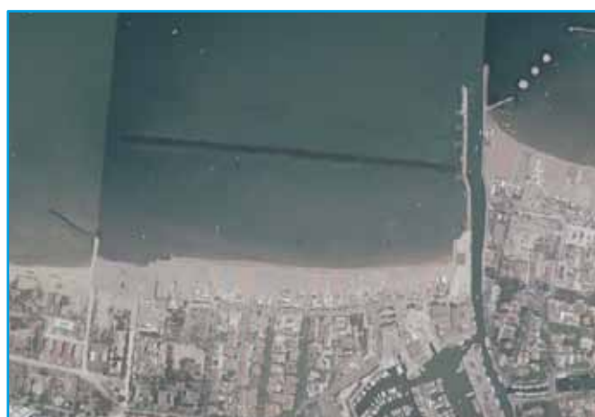
Figure 111. The semi-submerged breakwaters north of Cesenatico jetty harbour (March 2007).
