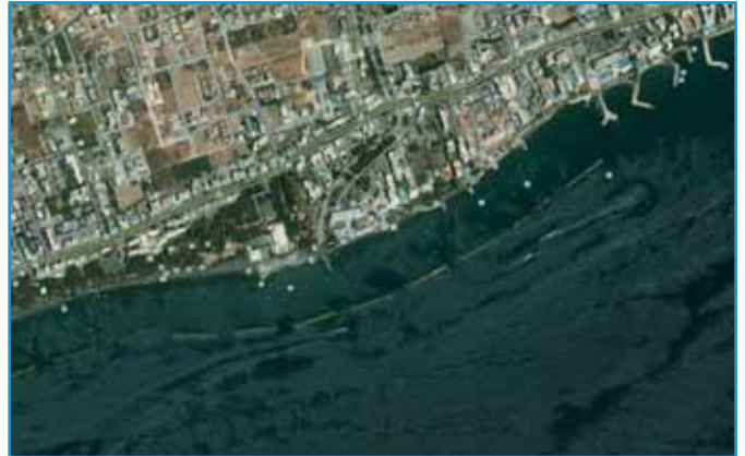
Figure 56. The same part of the Limassol waterfront on July 2008 (from GoogleEarth). The individual groynes have been replaced by detached breakwaters.
