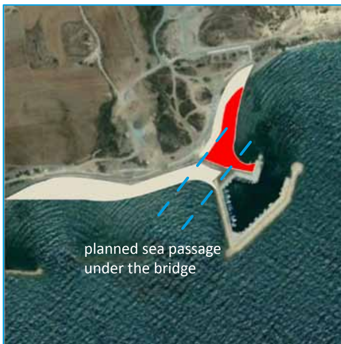
Figure 76. Sketch of the positioning of the excess sediment near the Alaminos Marina. In red the positioning of excessive sand that has to be removed so that the external docks of the marina to become operational again.
