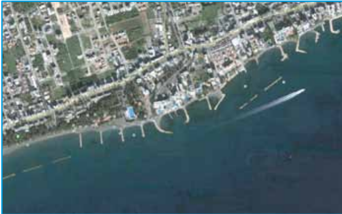
Figure 55. A part of the Limassol waterfront on January 2003 (from GoogleEarth). The individual groynes interrupt the seafront.
