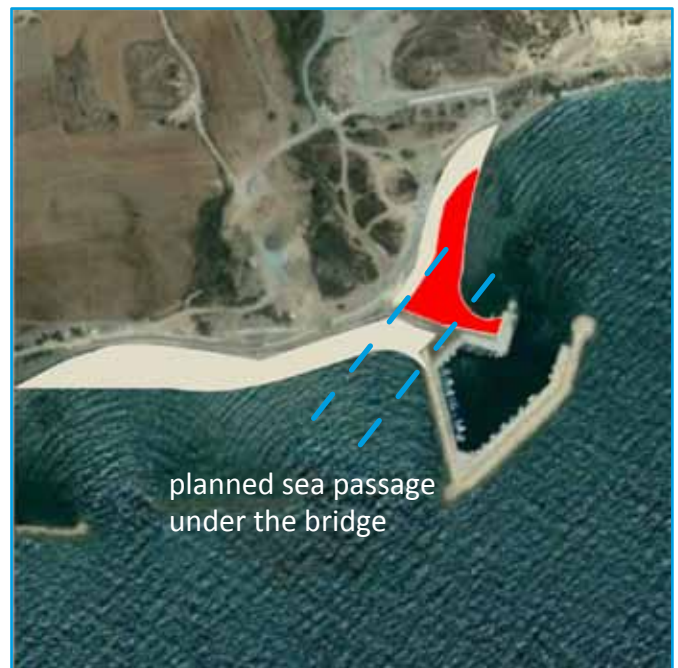
Figure 70. Sketch of the positioning of the excess sediment near the Alaminos Marina. In red the positioning of excessive sand that has to be removed so that the external docks of the marina to become operational again.
