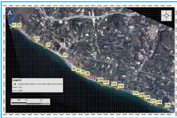
Figure 20. A: The intersection of the coastlines of years 1931 and 2009, define the nodal points C1 to C28 and 27 sedimentary sub cells. B: The intersection of the coastlines of years 1931 and 2009, define the nodal points C1 to C28 and 27 sedimentary sub cells.
