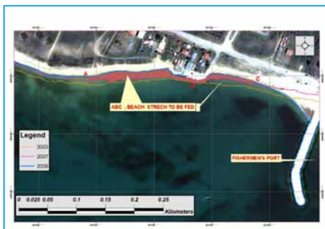
Figure 26. The critical coastal stretch which is taken as pilot case to be fed with sediment (marked with the letters ABC). Length 300 m, area 3,000 m 2 and mean width 10 m. Volume of sand for beach nourishment 30,000 m 3 .
